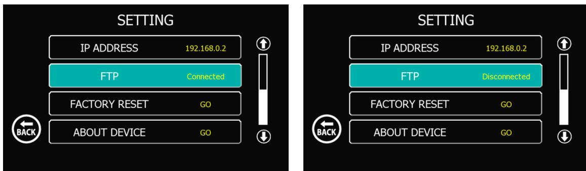
When connection with the FTP server was lost due to network problem or other reasons, event recording video and log file transmitted to the FTP server will be kept by HEV-1000 and it will start transmitting again when connection is back (Save/Transmit maximum 100 recordings)
